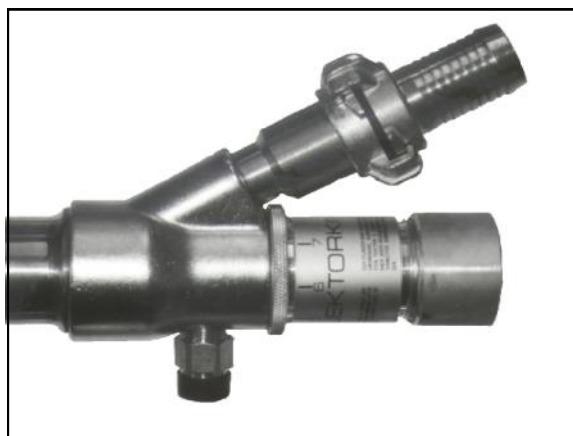
INJEKTORKING VARIO TURBO/COMBI with steplessly variable adjustment of the air volume and with quick clamp for the material hose.
