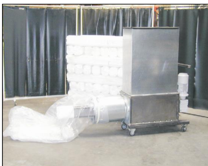
Styropactor MINI 1-PHASE with compacted pieces stacked on a pallet.
